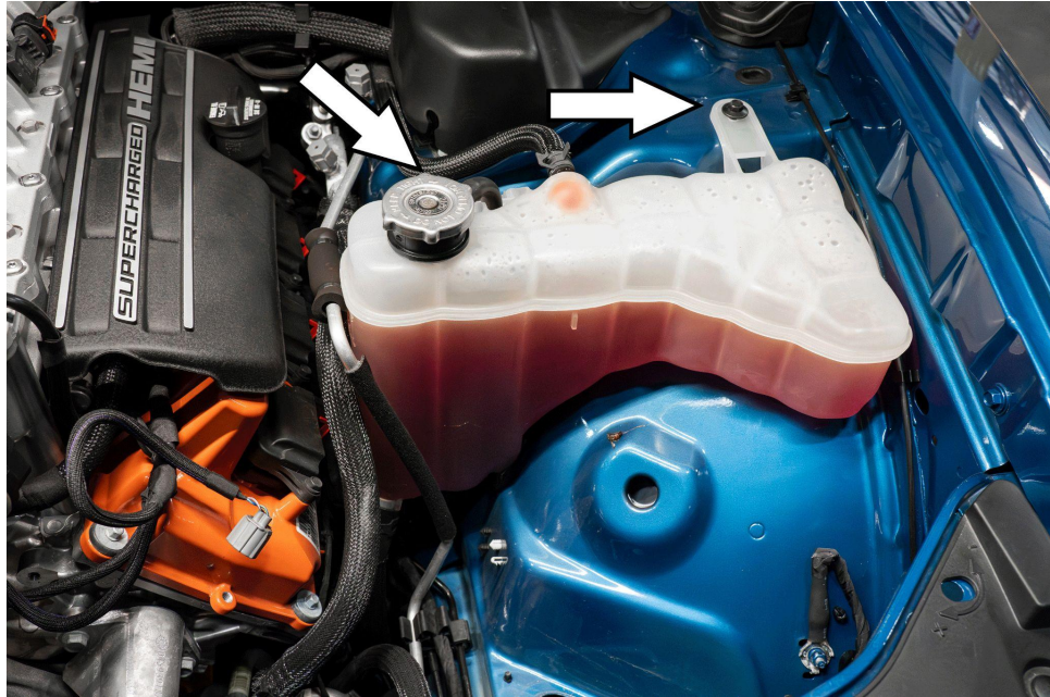
11. Reinstall the two 10mm bolts securing the coolant reservoir.
