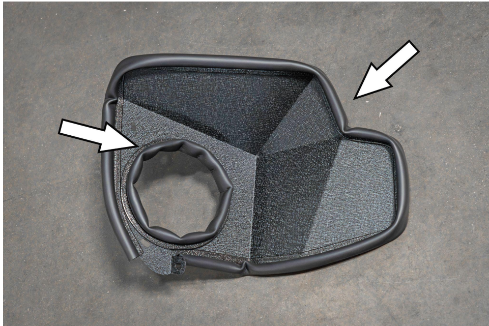
12. Install the provided bubble edge trim onto the heat shield as shown.
