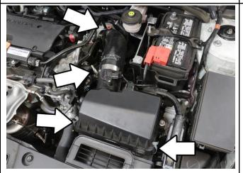
8. Insert the HPS silicone intake onto the throttle body and adjust the hose to the proper placement. Clip on the retaining clips securing the air box when the intake hose has been adjusted. Tighten the T-bolt clamps. **DO NOT EXCEED 15 INCH LBS.**
