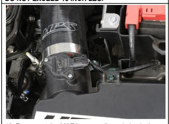
10. Reconnect the MAF harness clip and plug in the MAF harness connector back into the sensor.
