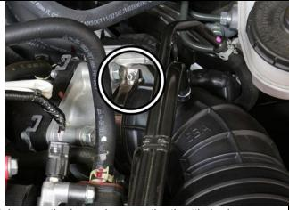
5. Loosen the hose clamp on the throttle body.
