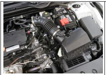
6. Remove the top portion of the air box along with the intake tube from the vehicle.
