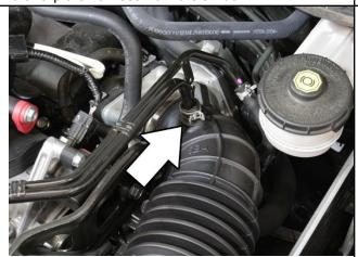
4. Disconnect the breather pipe from the intake tube.
