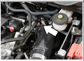
9. Insert the breather tube into the silicone intake.
