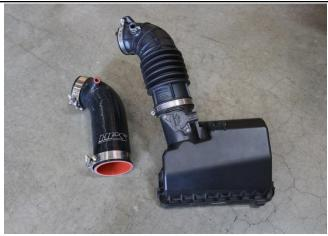
7. Remove the stock intake tube from the air box. Loosely install the T-bolt clamps onto the HPS intake hose, then insert it onto the stock air box.
