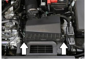
3. Unclip the retaining clips holding the top portion of the air box.
