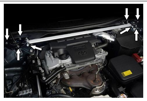
3. Install the strut bar assembly using the provided (6) M10 flange nuts. Then, tighten the preinstalled nuts and bolts holding the strut bar and the strut bar brackets together.
