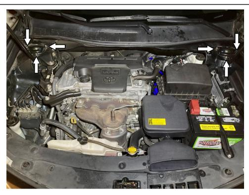
2. Loosen the (6) strut tower bolts.
