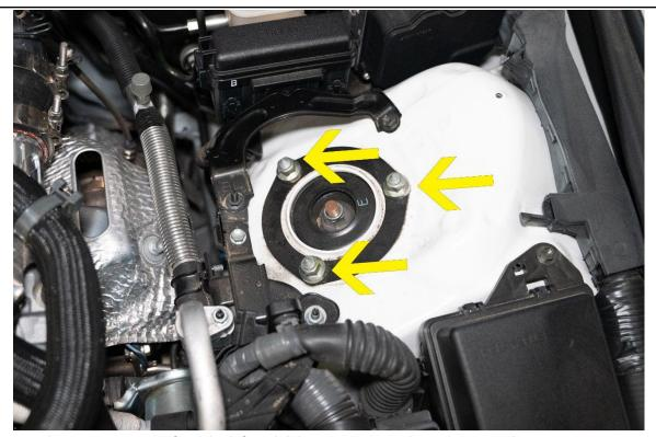
3. Remove the strut tower nuts from the left and right strut towers using a 14mm socket.
