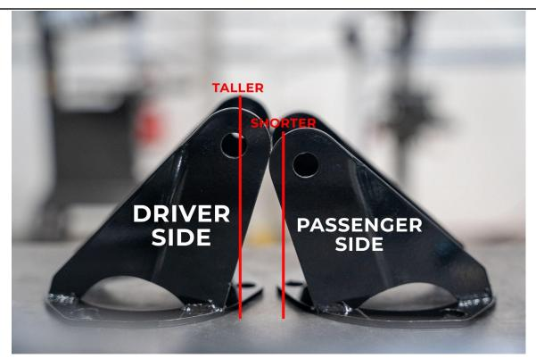
2. Identify strut tower brackets from left and right or driver side and passenger side. The driver's strut tower bracket is taller than the passenger's side strut tower bracket.
