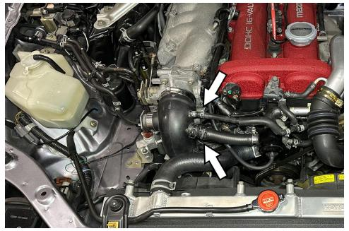
3. Disconnect the vacuum hose and the blow off valve recirculation hose. Once disconnected, remove the factory throttle body intercooler pipe.
