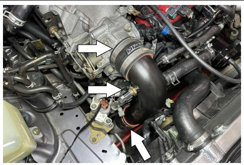
6. Slip the HPS intercooler pipe with couplers over the throttle body and lower intercooler pipe before tightening all four clamps. Install the intake air temperature sensor onto the HPS pipe using the original crush washer and then plug in the sensor harness.
