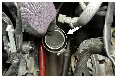
5. Loosely place the clamp onto the lower intercooler pipe. This clamp will be tightened once the HPS intercooler pipe is in place.
