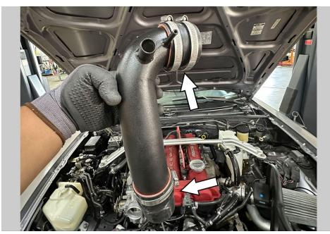
4. Install the straight coupler onto the short side of the HPS intercooler pipe and the reducer coupler onto the long side.
