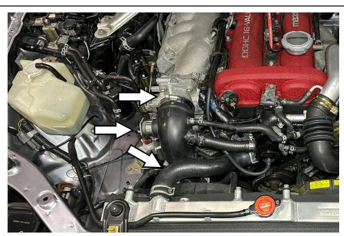
2. Loosen the top and bottom factory throttle body intercooler pipe clamps. Then unplug the intake air temperature sensor.
