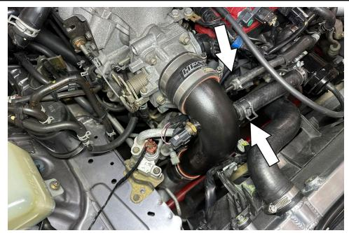
7. Connect the vacuum hose and the blow off valve recirculation hose to the HPS intercooler pipe.
