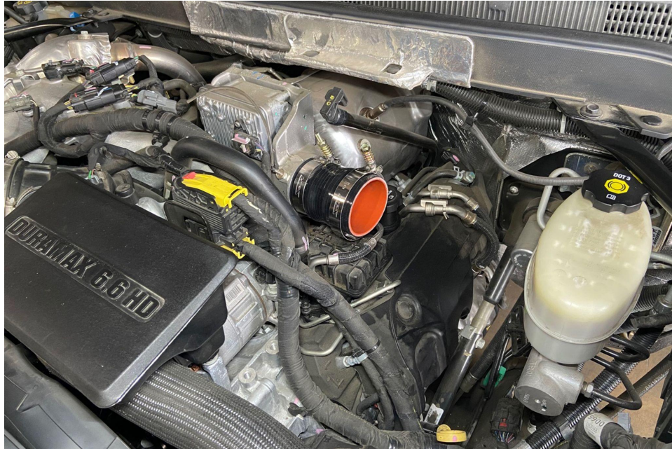
7. Install the silicone reducer onto the turbo outlet and secure it with the provided clamps.
