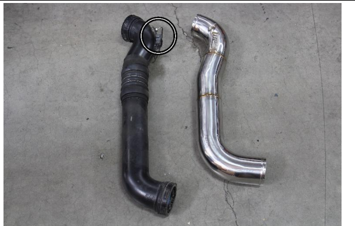
13. Remove the temperature sensor from the factory charge pipe to the HPS charge pipe.
