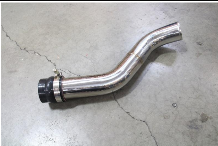
24. Install the hump coupler onto the long side of the hot side charge pipe.
