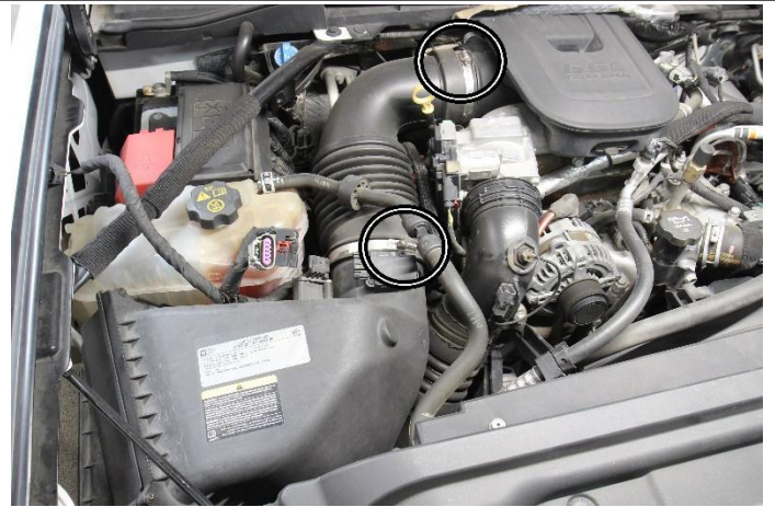
3. Loosen the hose clamp securing the factory hose from the air box and the turbo inlet.
