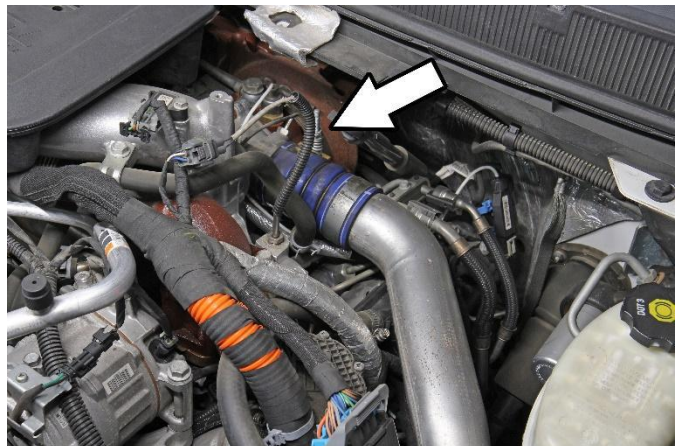
19. Loosen the hose clamp securing the hot side charge pipe from the turbo outlet.
