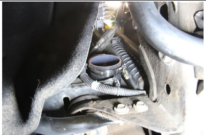
23. Install the other reducer coupler, along with the provided t-bolt clamps onto the intercooler inlet.
