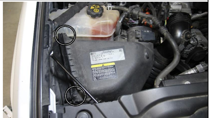
5. Loosen the two bolts securing the upper air box assembly.
