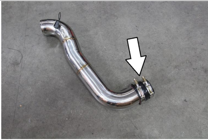
14. Insert the provided silicone reducer coupler along with the t-bolt clamps onto the end of the charge pipe indicated above.
