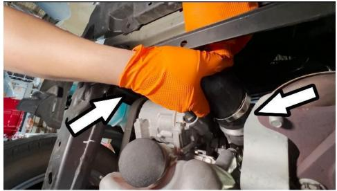
3. Locate the hot side intercooler hose located near the oil filter. Loosen the hose clamps securing the hot side charge hose from the turbo outlet and the intercooler. Remove the factory charge hose from the vehicle.
