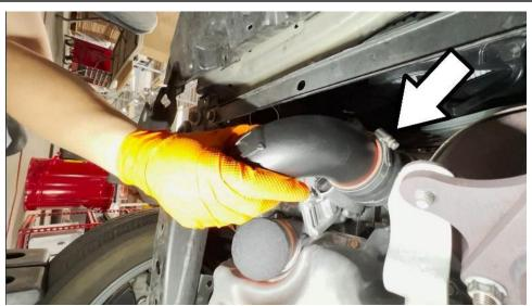
4. Insert and secure the hump couplers onto the turbo outlet and the intercooler along with the provided EMSC clamps. Insert the HPS charge pipe into the turbo side first, then into the intercooler side.
