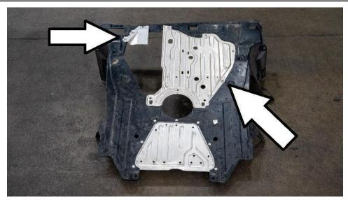
3. Loosen the 9 screws to remove the two pieces of aluminum undertray located under the vehicle.
