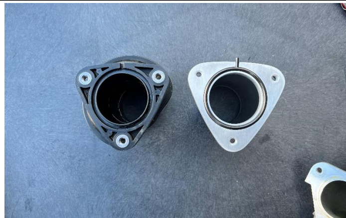
14. Remove the factory O-ring from the resonator and transfer it onto the HPS Resonator Delete.
