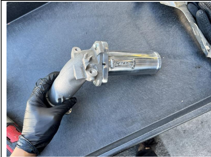
15. Secure the HPS Resonator Delete onto the turbo outlet elbow using the factory bolts. Torque to 8 ft-lb.
