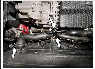
7. Loosen the hose clamp securing the intercooler hose from the intercooler inlet and disconnect it from the intercooler. Use a flat head screwdriver to release the electrical harness from the bracket then unclip the coolant hose from the plastic bracket.
