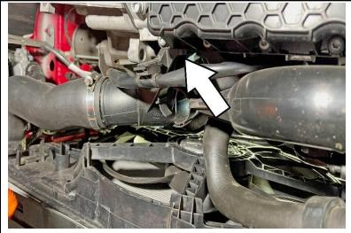
8. Loosen the T30 torx bolt securing the charge pipe bracket to the engine. Remove the hot side charge pipe from under the vehicle.
