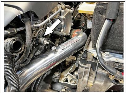
13. Carefully insert the hot side charge pipe from under the vehicle and into the coupler. Install provided 1" vibration mount onto the factory charge pipe mounting thread.
