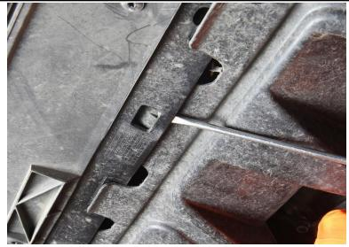
4. Using a flat head screwdriver, release the two tabs securing the lower engine cover and remove the panel from the vehicle.
