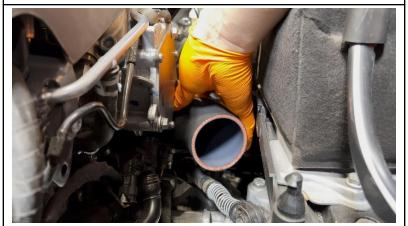
12. Insert the provided 45-degree coupler along with the provided clamps onto the turbo outlet. Do not tighten the clamp onto the turbo outlet at this time.
