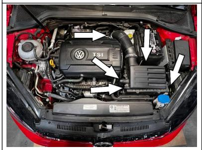
8. Disconnect the vacuum and SAI hose from the air box. Loosen the hose clamp securing the intake tube at the turbo inlet with a 7mm socket. Disconnect the intake tube then lift the air box assembly firmly to remove it from the vehicle.
