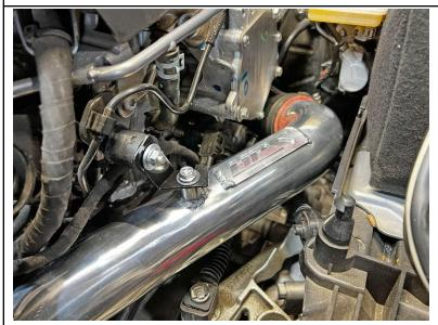
14. Use the provided M6 bolt, nut, and washers to secure the "L" bracket onto the vibration mount and charge pipe.
