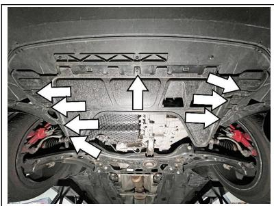
3. Remove the 8x T25 torx screws securing the lower engine cover panel.
