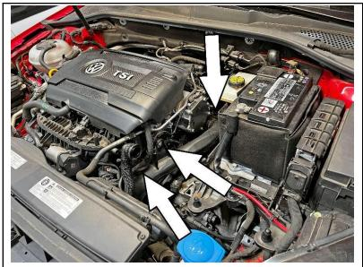
6. Unclip the wire looms from the front of the charge pipe then remove the T30 bolt securing the charge pipe to the engine. Loosen the hose clamp holding the charge pipe to the intercooler hose towards the rear of the engine, then disconnect the pipe from the intercooler hose.
