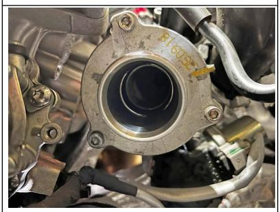
10. Remove the three allen bolts securing the turbo outlet muffler with a 5mm hex key.
