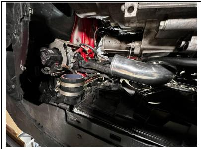
15. Insert the straight coupler along with the provided clamps onto the intercooler inlet.
