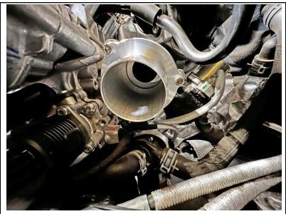
11. With the factory rubber O-ring is inserted and in the proper position, install the HPS outlet turbo muffler.
