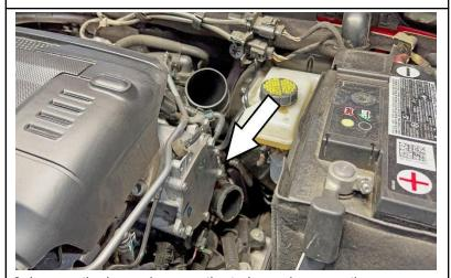
9. Loosen the hose clamp on the turbo and remove the intercooler hose from the vehicle.
