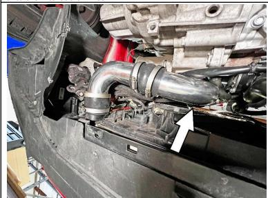
16. Insert the lower hot side charge pipe along with the provided hump coupler and clamps. Be aware of the clearance between the pipe and cooling fan. Secure all the clamps once everything is in position. Clip the coolant hose back into place.
