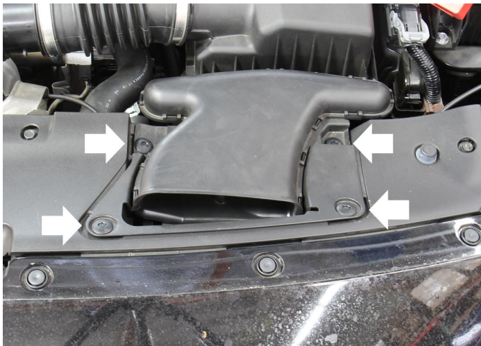
6. Push down the center of the 4 button clips to remove the air duct from the engine bay.
