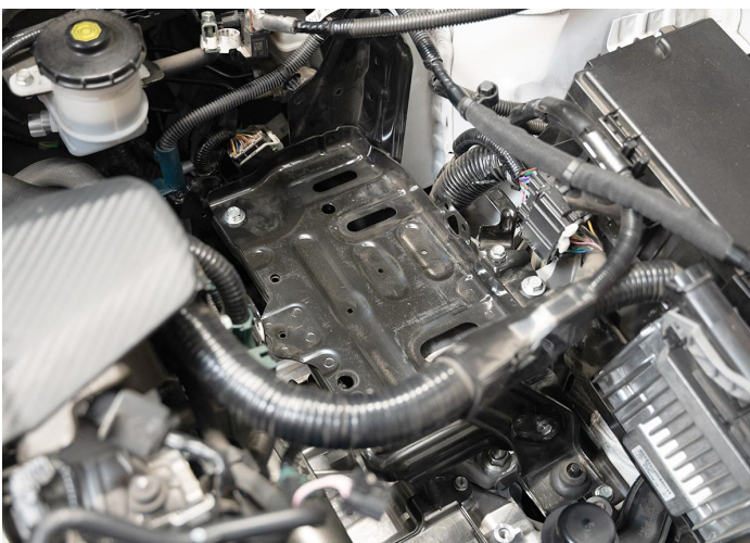
26. Reinstall the battery tray, battery, and intake system by reversing steps 2-11.
