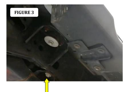
**Step-2** At the front location, you will need to drill the top hole. Continue threading a bolt plate in the guide bolt then introduce it through the obround hole, the tip of the bolt guide must come out through the top hole of the frame rail. Do not pull out the bolt plate attached to the bolt guide. (FIGURE 4).
