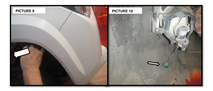
Release enough of the plastic clips holding your fender flare on to be able to pull it back and out of your way. You may remove this flare completely if you desire, but it is not necessary. (PICTURES 11 &12)
