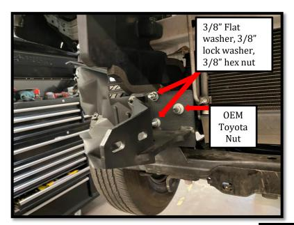
Install frame brackets. Reuse the OEM frame nuts on the larger threads (from page #. Use two 3/8" flat washers, two 3/8" lock washers and two 3/8 hex nuts to fasten the exposed studs on the bolt plate. Leave finger tight for final adjustment. Repeat process for both sides.
