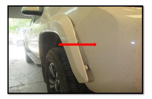
Once you are satisfied with the fitment of your bumper, you can cut the oem fender flares. Make a straight cut across so that the fender flare sits flush to the wings of the Element bumper. Use painters tape a guide.
