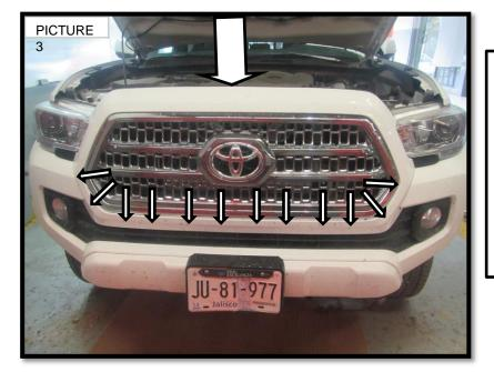
Begin the installation on the top of the vehicle, remove two grill screws (PICTURE 1). Remove two clip securing in back to the front grille. (PICTURE 2).
