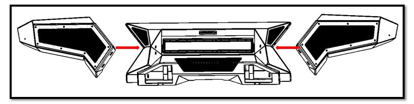
Install outer wings (without the mesh covers) onto the center section of the bumper. Exercise caution when installing each side to that you don't damage your paint. Each side with use four 3/8" hex bolts, four 3/8" lock washers, four 3/8" flat washers. This can be done with the mesh covers off as it will allow for greater access to the welded nuts on the center section.
