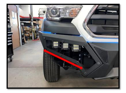
Once you have adjusted the fitment on your bumper, you can cut the fender liners. Depending on your desired look, you can cut the OEM fender liner by following the Element bumper lines. With caution, use a cutting wheel or box cutter to cut the inner fender liner. If you prefer to cut more material, please refer to the images below. You can sand the edges to so they are not left sharp.
