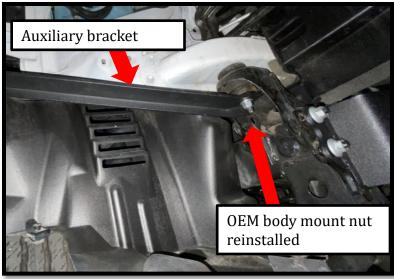
Install auxiliary bracket with the fold facing the tires (see image) and fasten the OEM body mount nut back in place. Leave finger tight to allow for final adjustment. For torque settings, please refer to your OEM repair manual.
