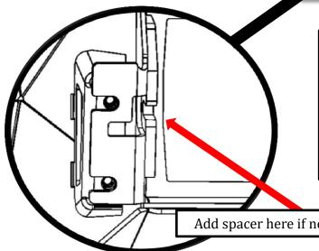
Depending on the light bar brand you decide to use, you may find that it will require spacers to fill in any voids. We supply 3/4" OD plastic spacers. They are to be installed on the backside of the bumper, where the might bar mount is located.
