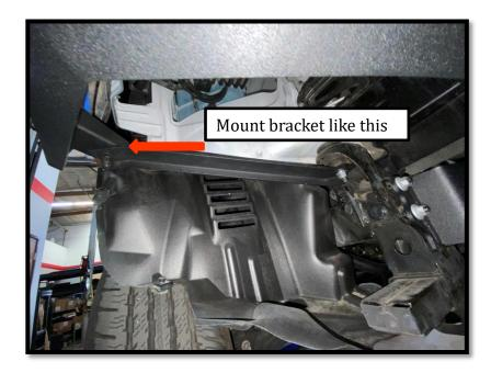
Once both wings are installed, connect outer auxiliary bracket to the outer part of the wing. The auxiliary bracket sits on the bottom of the welded bracket on the bumper wings. Use one 3/8" x 1 hex bolt, two 3/8" flat washer, one 3/8" lock washer and one 3/8 hex nut. Leave finger tight and repeat process for both sides.
