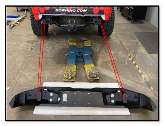
With assistance, position bumper onto OEM bumper mounts.
