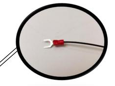
**Step 16:** The door trigger sensor harness will need a ground connection to the vehicle. Locate the seat belt assembly at the driver side b-pillar and install the ground wire under the top bolt of the seat belt assembly.
