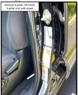
**Step 15:** Route the DRIVER side door trigger wire (brown) towards the DRIVER side b-pillar. Route the PASSENGER side door trigger wire (white) and the black disable switch wires under the center console to the left side of the vehicle. The white wire needs to go to the passenger side b-pillar, the black wires will go to the center console.
