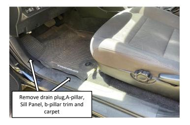
**Step 13:** On the DRIVER side, remove the front kick panel, front door sill trim panel and b-pillar trim panel. Go under the driver seat and locate the split in the carpet. Pull the rear half of the carpet back to expose the oval rubber drain plug. Pull the drain plug and drill a 7/16" hole.
