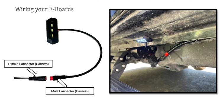
**Step 11**: Align the arrows on the small round connectors and plug the Driver side front and Driver side rear LED lights. Prepare the surface by cleaning with a 50/50 mix of isopropyl alcohol and water or equivalent. Once the surface is completely dry, peel the backing from the double-sided tape and stick the LEDs to the bottom side of the rocker panel. Position the LED lights at the center of the front and rear passenger side doors
