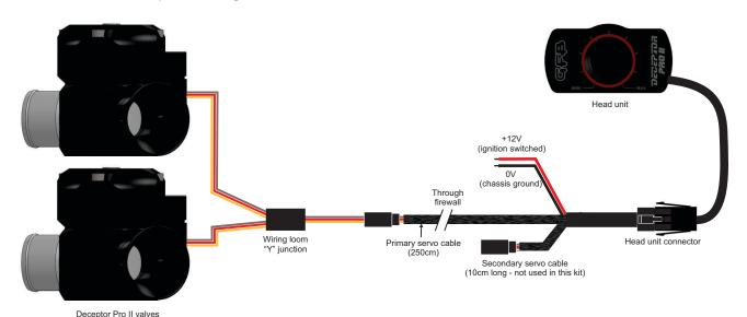
Continue the installation by feeding the primary servo cable through the firewall into the engine bay. Ensure that the cable is protected where is passes through the firewall to prevent shorting out.
