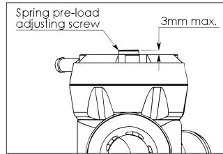
Take the car for a drive, and take note of how easily the valves vent when you lift off. Making the springs softer will allow the valves to open easier and vent longer, and increasing the pre-load means you will need to drive the car harder (i.e. more boost) before you start to hear the BOVs venting, and the blow-off sound will be shorter in duration.
