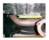
STARTING WITH THE REMOVAL OF STOCK MANIFOLD, REMOVE POSITIVE BATTERY CABLE IN THE ENGINE COMPARTMENT. NOW STARTING WITH THE DRIVERSIDE, REMOVE DRIVERSIDE HEADPIPE AND THEN REMOVE STARTER. FOR EASIER REMOVAL OF STOCK MANIFOLD AND INSTALLATION OF GIBSON **HEADERS NOW REMOVE** STOCK MANIFOLD AND HARDWARE MAKING SURE TO CLEAN HEAD SURFACE OF ANY DEBRIS, BEFORE INSTALLATION OF GIBSON HEADER.
