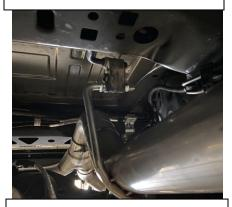
5. Install the y pipe and insert the hanger into the factory rubber grommet on the supplied Gibson hanger. Install the driver side pipe as well. Keep in mind the length the pipe is slid on will change the angle of the tip. Make adjustments until it fits correctly.
