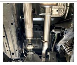
3. with Muffler in place install your over axle pipe. Keep everything loose until all is installed. Be sure to not bottom out the hanger into the factory grommet. It will create vibration.
