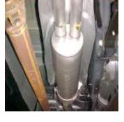
HEADPIPE 1 ½" TO 2". USE CLAMP # G TO SECURE MUFFLER TO HEADPIPE. DO NOT TIGHTEN. USE A JACK STAND TO HOLD UP THE MUFFLER. OUTLETS SHOULD BE LEVEL.
