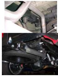
INSTALL PASSENGER SIDE TAILPIPE # C INTO MUFFLER 1 ½" TO 2". INSERT WELDED HANGER INTO RUBBER GROMMET, USE CLAMP # H TO SECURE PIPE TO MUFFLER. DO NOT TIGHTEN. ROTATE PIPE TOWARDS DRIVERSIDE.
