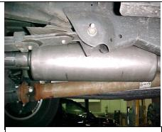
3 INSTALL MUFFLER # B ONTO HEADPIPE 1 ½" TO 2". USE CLAMP # F TO SECURE MUFFLER TO HEADPIPE. DO NOT TIGHTEN. USE A JACK
