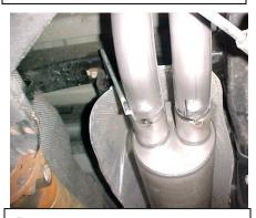
5. INSTALL DRIVERS SIDE TAILPIPE # D INTO MUFFLER 1 ½" TO 2". INSERT HANGERS INTO RUBBER GROMMETS, USE CLAMP # G TO SECURE PIPE TO MUFFLER. DO NOT TIGHTEN.
