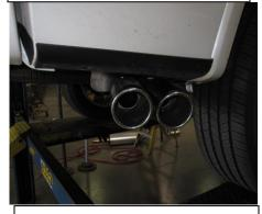
7. Be sure to check all clearance after each section has been tightened to be sure there is proper clearance. It may take 4-500 miles for your vehicle to fully adjust to the changes in exhaust flow.
