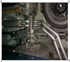
6. THE TAB ON DRIVER SIDE PIPE SHOULD GO UNDERNEATH THE PASSENGER SIDE PIPE TAB. USE BOLT KIT # H TO SECURE TOGETHER.
