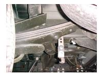
NEXT INSTALL DRIVERS SIDE OVERAXLE PIPE #D INTO MUFFLER 1 ½" TO 2". USE CLAMP #I TO SECURE PIPE TO MUFFLER. DO NOT TIGHTEN. ROTATE PIPE UNTIL IT TOUCHES HANGER. USE CLAMP #I TO HOLD PIPE TO HANGER DO NOT TIGHTEN.
