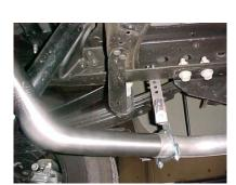
INSTALL PASSENGER SIDE OVERAXLE PIPE #C INTO MUFLER
