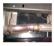
LAY OUT THE GIBSON EXHAUST ON THE FLOOR SO IT LOOKS LIKE THE DRAWING. COMPARE PART NUMBERS WITH MANUAL. TO REMOVE YOUR STOCK EXHAUST, REMOVE IT FROM THE CLAMP LOCATED JUST IN FRONT OF THE MUFFLER. YOU MAY NEED TO HEAT IT UP FOR EASIER REMOVAL. NOW CUT OFF YOUR STOCK TAILPIPE JUST BEHIND THE MUFFLER. USE WD-40 TO AID IN THE REMOVAL OF HANGERS. LEAVE ALL RUBBER GROMMETS IN PLACE.
