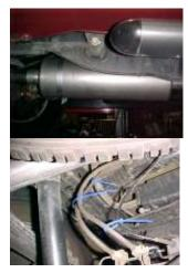
MAKE SURE YOU HAVE A 1" CLEARANCE ON ALL RUBBER BRAKE LINES, SHOCK BOOTS, TIRES, FUEL LINES, ETC...
