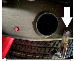
5. Install the Driver side hanger into the factory existing hole in frame. Install the Driver side pipes. Keep everything loose until everything is installed.
