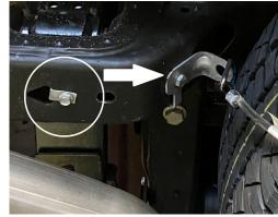
4. Relocate the the factory spare tire cable bracket to ten hole closer to the spare tire using bolt kit # L. You can install the passenger side overaxleipe. Note all hangers will sit in the rubber hangers level.
