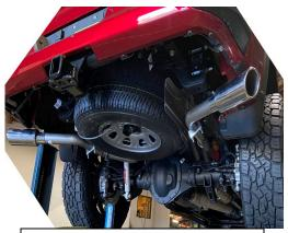
6. With proper clearance from spare tire, install the exhaust tip onto the tailpipe. The system was designed to have the tip 1" below the quarter panel of the vehicle. Note you can adjust the tip position inward or outward with rotation of the exit pipes.
