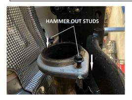
2 First you'll need to unbolt the factory flange and remove the exhaust. Next, hammer out the studs protruding from the factory flange, then install head pipe #A and tighten with allowance for adjustment using Bolt Kit #M.
