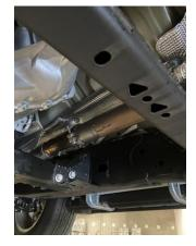
3. INSTALL HEADPIPE #A ONTO STOCK PIPE. INSERT WELDED HANGER INTO RUBBER GROMMET. (You Will be reusing the factory head pipe clamp.)
