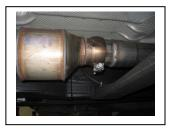
4. Install head pipe #A onto factory pipe re-use your factory clamp to secure insert welded hanger into rubber grommet. Do not tighten
