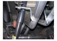
5. Make sure muffler outlets are level before installing tailpipes. Now install passenger tailpipe #C. Insert welded hangers into rubber grommets.
