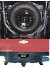
8. Install exit pipes #E onto tailpipes. Cut to your preferred length then use clamps to secure exit pipes to tailpipes. Install stainless steel tips. Clamp down.
