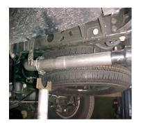
INSTALL EXIT PIPES # E. USE CLAMPS # G TO SECURE TO THE TAILPIPES. DO NOT TIGHTEN.
