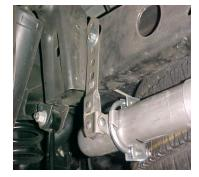
INSTALL METAL HANGER # I INTO HOLE LOCATED APPROXIMATELY 23" FROM THE REAR OF THE FRAME. USE TOP HOLE ON HANGER. INSTALL DRIVER SIDE OVERAXLE TAILPIPE # C INTO THE MUFFLER 1-1/2"-2". USE CLAMP #H TO SECURE PIPE TO MUFFLER.DO NOT TIGHTEN.
