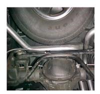
INSTALL THE PASSENGER SIDE OVERAXLE TAILPIPE #D TO THE MUFFLER 1-1/2"-2". USE CLAMP # H TO SECURE TAILPIPE TO MUFFLER. DO NOT TIGHTEN.
