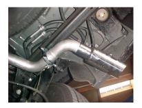
USE CLAMP # I TO SECURE TO THE MUFFLER, INSERT WELDED HANGER INTO THE RUBBER GROMMET. DO NOT TIGHTEN. NEXT, INSTALL THE EXIT PIPES # E, USE CLAMPS # H TO SECURE TO THE TAILPIPES. DO NOT TIGHTEN.
