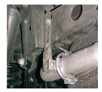
INSTALL METAL HANGER # J INTO HOLE LOCATED APPROXIMATELY 17" FROM THE REAR OF THE FRAME. USE TOP HOLE ON HANGER. INSTALL DRIVER SIDE OVERAXLE TAILPIPE # C INTO THE MUFFLER 1-1/2"-2".
