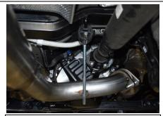
3. Install your Driver side head pipe #A using the factory Gasket and supplied bolts in Item #K and install your Passenger side headpipe. Do no tighten until final install.
