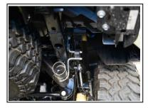
6. Install the Passenger overaxle pipe (E) using clamp (H) and hanger assembly (I). Use one of the body bolts (as shown in picture) and rubber grommet(K). Do not tighten.
