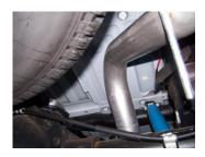
6. Slide the over axle tailpipe #C into the muffler 1.5-2". Use clamp #E to secure tailpipe to muffler. Do not tighten. Insert welded hangers into rubber grommets.
