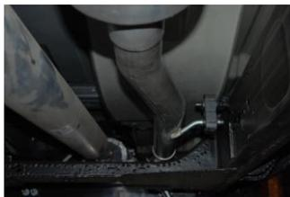
Next, install headpipe #A into adapter #N. Insert welded grommet. Use clamp #F to secure, do not tighten.
