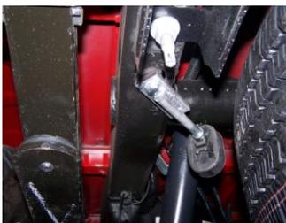
5. Install metal hanger #H into hole located approximately 16" from the rear of the frame. Use hardware kit #I, washer #M, and rubber grommet #J.
