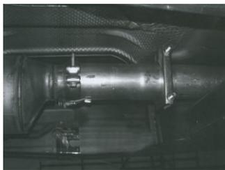
3. Bolt adapter pipe #N to the stock flange re-using the factory clamp.
