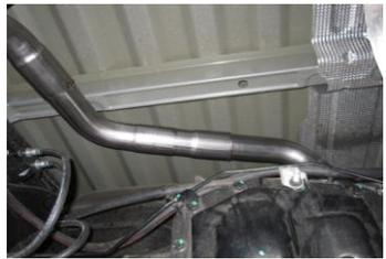
6. Install driver side tailpipe #C into muffler 1.5-2". Rotate until it touches the rear mount, use clamp #H to secure tailpipe to muffler. Do not tighten.
