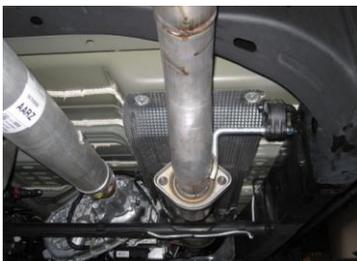
3. Install headpipe #A onto your existing stock 2-bolt flange. Use your factory nuts. Insert hanger into rubber grommet. Do not tighten. **On short beds cut 12.5" headpipe**
