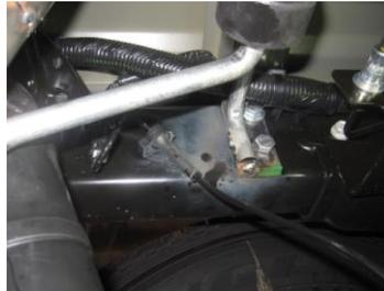
5. Install the driver side rear tailpipe hanger #F onto frame using bolt kit provided.
