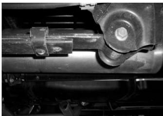
4. Slide muffler #B onto headpipe 1½"-2" with the louvers facing towards the converter. The muffler outlet should be positioned at 12 o'clock. Use a jack stand to support the muffler. Use clamp #E to secure the muffler to the headpipe. Do not tighten. Muffler inlet is looking into the louvers.
