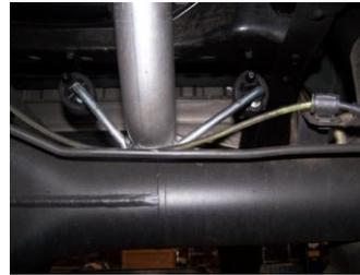
5. Slide the over axle tailpipe #C into the muffler 1½"-2". Insert welded hangers into rubber grommets. Use clamp #E to secure the muffler and tailpipe together. Do not tighten.
