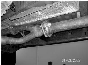
2. To remove the stock exhaust, unbolt it at the 2-bolt flange located in front of the muffler. Disengage hangers from OEM rubber grommets. Use WD-40 to aid in this process. Do not damage or remove the OEM rubber grommet as you will reuse them to mount your new system.
