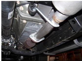
3. Install headpipe #A at the 2-bolt flange connection. Secure with bolt kit #F. Do not tighten. Insert welded hanger into rubber grommet.
