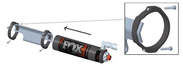
Fig. 4: Remote reservoir and bracket assembly.
