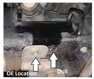
Fig. 2: The OE radiator bracket is used to mount the reservior bracket.
