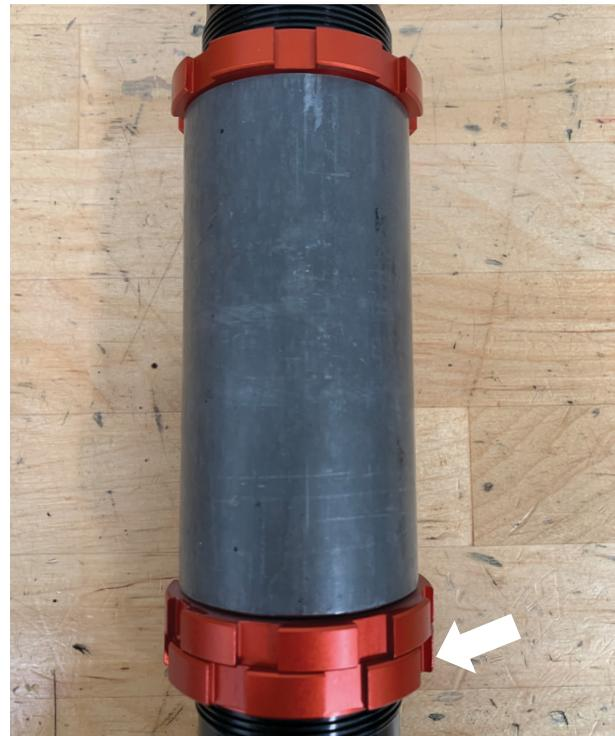
Fig. 7: The third lock ring acts as a jam nut.
