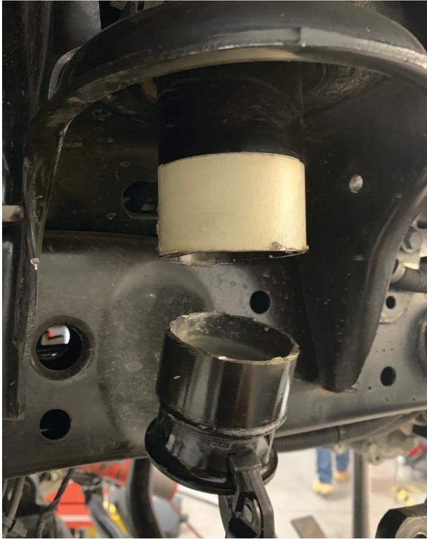
Fig. 2a: Cut the bump holder off under the tape line. Passenger side shown.
