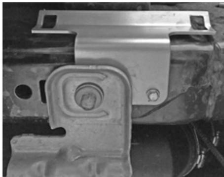
Fig. 3: Driver side Reservoir Bracket
