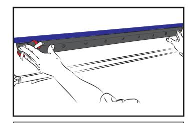
**STEP 4:** Aligning the rear end of Body Side Moldings with the position noted in step 2. Position the Body Side Molding so the top edge of part is running parrel along the base of the ridge line profile in the door surface. Ensure the tape liner along top, bottom and ends are on the ouside edge of Body Side Moldings.
