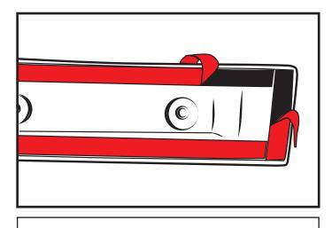
**STEP 3:** Peel back approximately 2" inches of protective tape liner and fold to the outside of Body Side Moldings at a 45 degree angle along top, bottom and ends of Body Side Moldings. **Important: Do not touch the exposed surface of the tape.**
