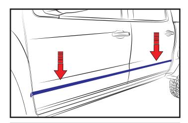
**STEP 1:** Clean the door areas where the Body Side Moldings will make contact with the door surface. Ensure doors are dry prior to install. Apply masking tape to front and rear doors along the top of the ridge line in the door profile. Ensure the masking tape is in a straight line to assist with aligning the Body Side Moldings to the front and rear doors.
