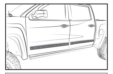
**STEP 7:** Remove masking tape from door surface. Repeat the previous steps for opposite side of vehicle to complete installation of Body Side Moldings.
