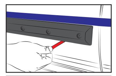
**STEP 5:** Ensure Body Side Molding is positioned correctly on the door surface before applying light pressure to the exposed tape areas. Slowly peel the remaining tape liner away by pulling on the exposed ends of liner and apply firm pressure around the attachment areas.
