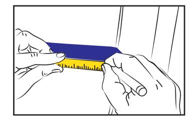
**STEP 2:** Using a ruler measure in 2 cm inch from the back end of front and rear doors marking the position with a non-permanent marker on masking tape. Ensure the correct Body Side Moldings are identified prior to installing to front and rear doors. Parts are identified on the back side of Body Side Moldings.
