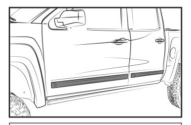
**STEP 7:** Remove masking tape from door surface. Repeat the previous steps for opposite side of vehicle to complete installation of Body Side Moldings.
