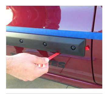
**STEP 5:** Ensure Body Side Molding is positioned correctly on the door surface in the desired location. Slowly peel the remaining tape liner away by pulling on the exposed ends of liner and apply firm pressure around the attachment areas.
