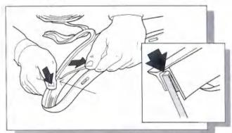
4. Pulling at right angles to the extrusion, remove the liner from the extrusion in small portions and apply
