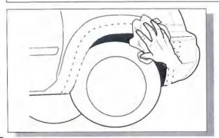
Wash the areas of contact on the vehicle and wipe dry both the vehicle and the Fender Flares with a clean cloth. Ensure inside of Fender Flares where extrusion is attached is clean, use alcohol wipe supplied to clean surface.
