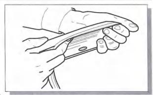
3. Remove approximately 2" (50mm) of the protective liner from the extrusion. Fit the extrusion to the Fender Flare along the edge that comes in contact with the vehicle's body panel.
