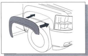
7. Place the front Fender Flares onto the vehicle and line up the holes on the part with those of the screw holes on the vehicle.
