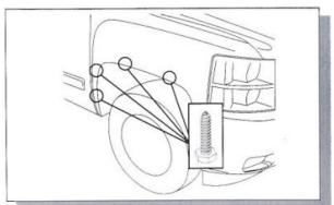
6. Use the original manufacturer's hardware that is in the wheel arch of the vehicle to fit the Fender Flares. Remove the 7mm socket head screws from the fasteners on the vehicle.
