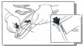
5. Pulling at right angles to the extrusion, remove the liner from the extrusion in small portions and apply thumb
