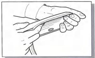
4. Remove approximately 2" (50mm) of the protective liner from the extrusion. Fit the extrusion to the Fender Flares along the edge that comes in contact with the vehicle's body panel, ensuring the double sided tape is being adhered to the inside surface of the fender
