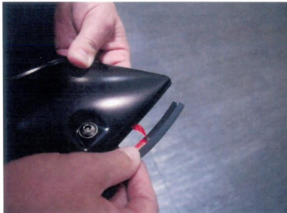
**STEP 1:** Attach the included rubber seal to the Fender Flares by peeling back 2" of the adhesive liner and position so the double sided tape adheres to the inside of the Fender Flare. Attach rubber seal to top leading edge of part that will make contact with the vehicle body.
