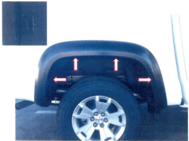
**STEP 6:** Place the Fender Flare onto the vehicle in position of best fit following the contours of the body. Use (4) of the U-style clips to secure the Fender Flare to the vehicle body. Make sure the barb in the clip securely attaches in the slot on the Fender Flare.
