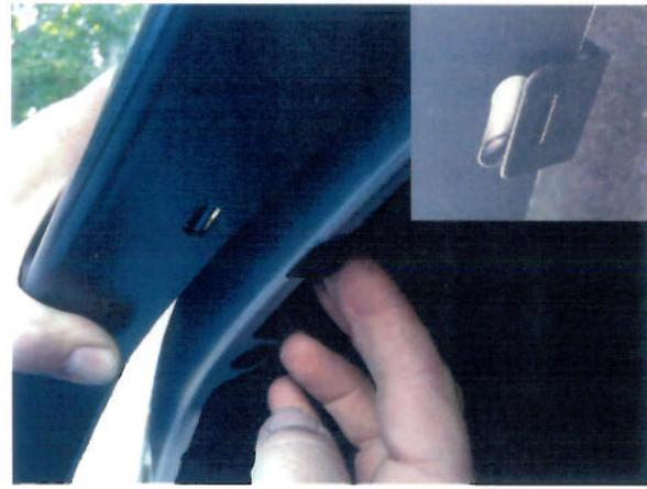
**STEP 6:** Place the Fender Flare on the vehicle in the position of best fit. Locate the 2 mounting slots at the top of the Fender Flare and use 2 of the U-style clips to attach. It is critical to first place the clips onto the wheel arch sheet metal (as shown) and then slide the product into position be engaging the barb in the clip into the slots on the Fender Flare.
