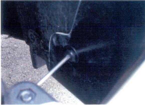
**STEP 7:** Reinstall the #15 Torx head screw, removed in STEP 5, back into the the lower rear section of the Fender Flare.
