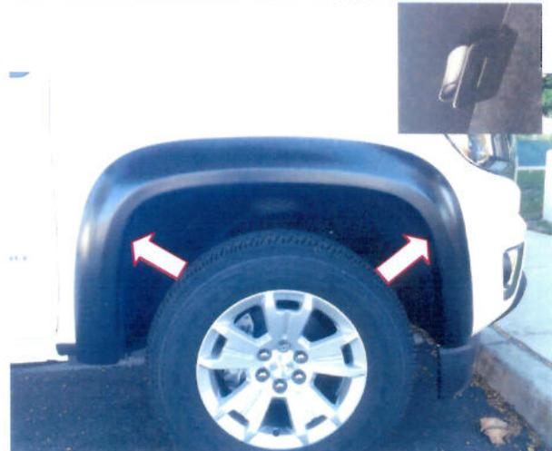
**STEP 10:** Secure the remaining "U" style clips at the vacant slots and repeat for opposite side. Double check all hardware is tight and rubber seal is flat/firm against vehicle.
