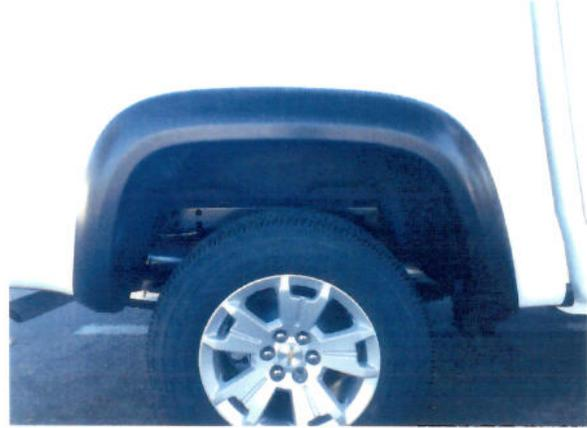
**STEP 8:** Repeat installation method for opposite side. Double check all hardware is tight and rubber seal is flat / firm against vehicle surface. Do not use abrasive cleaners.
