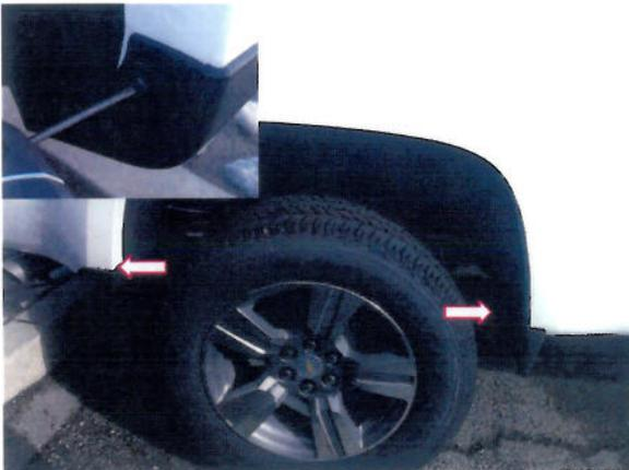
**STEP 5:** Locate the 2 outer screws. Remove the screws using a #15 Torx head screwdriver. Retain screws for later re-installation.
