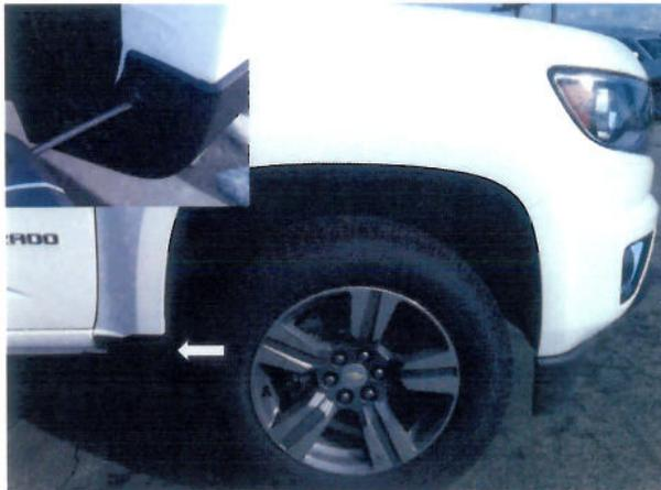
**STEP 5:** Locate the #15 Torx screw at the lower rear section of the wheel well and remove the Torx screw. Retain the screw for later re-installation.
