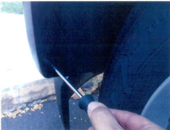
**STEP 9:** Use the screw and washer to secure the front of Fender Flare to the vehicle body.
