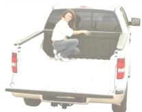
While temperature does not affect your DualLiner, it is easier to install when the bedliner is above 50 degrees Fahrenheit. If working in colder temperatures, it is helpful to warm the bedliner indoors prior to installation. The mat may take a "set" while rolled. If possible, unroll the mat and let it "relax" in the sun to make it easier to work with. If installing in cold weather it may take several weeks for the mat to fully relax.
