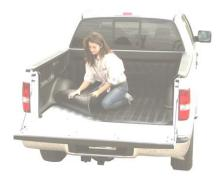
With the mat in, you can start reinstalling the tie-down cleats and BoxLink plates. Start by finger-tightening all locations that will allow the panel to be moved back and forth or up and down to properly install. Take care not to over torque or overtighten – these are aluminum beds. The rear of the sidewall panels, near the tailgate where the tie-down cleats with T40 bolts is located should be pushed all the way to the surface of the truck for a tight fit.
