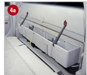
Rotate jack so yellow knob faces outward (as pictured).
