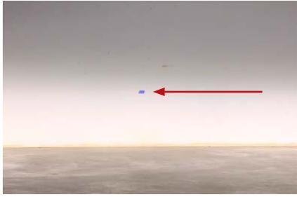
14. Aim your SS3 pods on each side, so that the top of the beam pattern is on the cutoff line mark.
