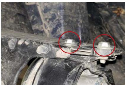
5. Pull the fender liner back and remove the two 10mm bolts holding the factory fog lamp in place. Remove the factory lamp.
