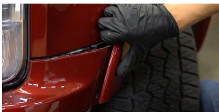
4. Using a plastic trim removal tool, loosen the upper bumper piece. Repeat the steps on the other side of the vehicle to remove the upper bumper piece from the vehicle.
