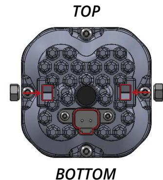
1. Install the supplied nuts into the pod housing with the nylon facing inward. Attach the bracket to the pod using the supplied screws and washers. Make sure the bracket is in the correct orientation. There will be a small gap between the pod and bracket to allow for aiming. See diagrams above. Ensure that the screws are tightened such that the pod retains its position, but can pivot with force for aiming.
