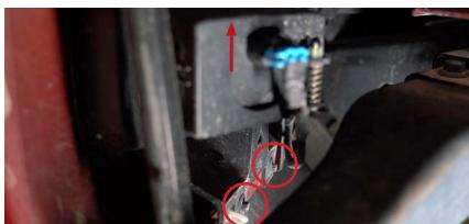
6. Remove the fog light bezel from the bumper, by removing the three 8mm bolts holding it in place and disconnecting the fog light harness. If applicable, remove the two 13mm bolts holding the bracket blocking the fog light bezel in order to gain access to the fog light bezel.
