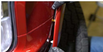
3. Peel the plastic fender flare back using a plastic trim removal tool. Loosen the plastic clips holding it in place using a pick tool.
