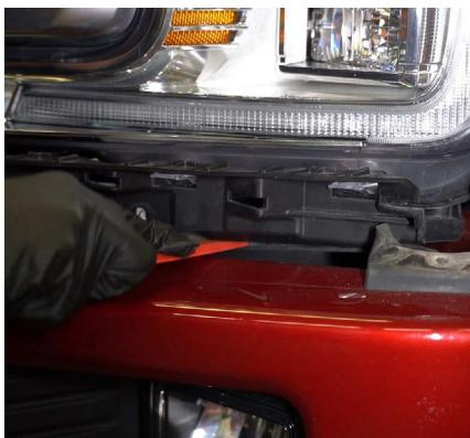
5. Remove the shroud blocking access to the fog light bezel. To do so, remove the 10mm bolt and loosen the three plastic pins holding the shroud to the bottom of the headlight. Then remove the two 10mm bolts near the fender flare. Remove the shroud from the vehicle.
