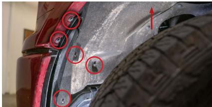
2. Peel back the wheel well fender liner. To do so, remove the two push clips, two 5.5mm bolts, and two 7mm bolts shown in the picture to the left and peel the fender liner back.
