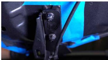
4. Slide the ditch light bracket under the hinge and align the holes with the hood hinge. Adjust the bracket to leave a slight gap at the back of the hood before tightening.
