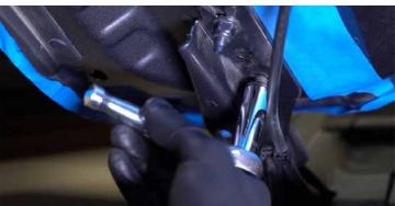
3. Loosen the two 13mm bolts securing the hood hinge, while holding the back of the hood. Work on one side of the vehicle at a time to minimize movement of the hood.
