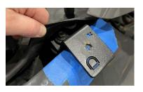
3. Install your new ditch light bracket using the factory fender bolt. Place the bracket as close to the fender as possible without touching the fender. Ensure that the top of the fender lines up well with the hood and A-pillar after install.
